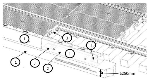
RUBBER EDGE BEAMS ON CONCRETE SILL BEAMS, SET ON COMPACTED CONCRETE BED & SUB-BASE AS SPECIFIED BY CLIENTS OR INSTALLERS CIVIL ENGINEER.
